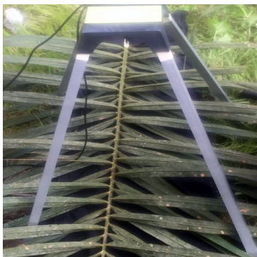
Figure 12. Camera distance controlled for better detection. Image by Najib et al. (2021b).
